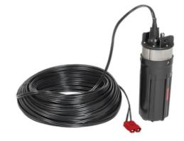
The Engineered Plastic 12-volt Abyss 300® pump is capable of pumping up to 300 feet depth to water (DTW) by simply connecting the Abyss 300® to a 12-volt deep cycle battery using the Low Flow with Power Booster 4 Controller. Its reliable design and low amp consumption makes it the ideal pump for groundwater sampling and remediation pump and treat system.
